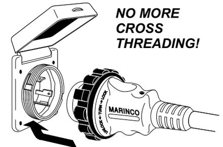
To use the Easy Lock System, align the lock locator tabs on the Easy Lock ring on the cordset with the slots on the sides of the threaded boss on the inlet. Push the Easy Lock ring onto the boss and twist 1/8 turn for a positive water-proof connection.
