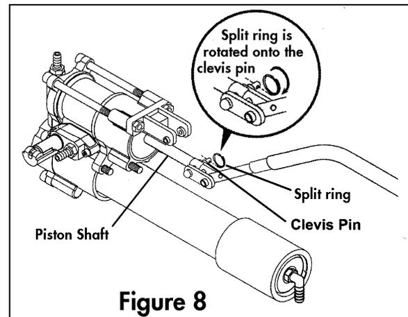
9. Operate the pump handle back and forth through its full range of travel in both directions. Pump at a rate of approximately one complete cycle every two seconds (one second in each direction). This is about the same rate at which the pump is driven by the motor during powered operation. Do not pump too fast!
