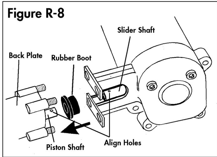
10. Slide the two 5" sockethead capscrews through the holes in the check valve plate and the back plate. Slide the rubber boot onto the piston shaft. See **Figure R-8**.
