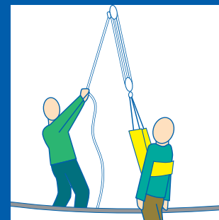
Fig. 19 Hoist COB aboard
