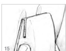
oxy thickened with adhesive filler is difficult to sand. Wet sand with 80-120-grit wet/dry sandpaper (15).
