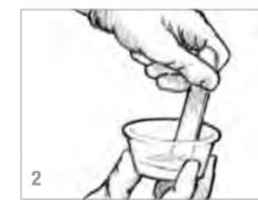
Each 105/205 packet in this kit contains the correct proportion of resin and hardener required to reach full cure. Be sure to squeeze out all of the contents of each resin/hardener packet you open.
