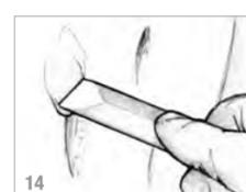
5. Fill the cavities with the thickened epoxy mixture using the flat end of the mixing stick (14).
