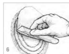
ing them evenly over the larger pieces (5). Mix more epoxy as necessary to saturate all layers of fiberglass in the void with epoxy. Allow the epoxy to cure until it begins to gel.
