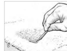
Coat the substrate with mixed 105/205 epoxy. Lay the fabric in position on the wet epoxy. Spread mixed epoxy onto the fabric using a glue brush. When the fabric and substrate have been saturated, use the side of the mixing stick as a squeegee to smooth and remove excess epoxy (8). Repeat the process with additional layers.
