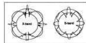
The best overall performance for the Davis was not in the often-recommended "catch rain" position, but in the "double catch-rain" position, which has the advantage of very little degradation of performance with heel. The average RCS was 5.0 m<sup>2</sup> upright, and 4.5 m<sup>2</sup> heeled 20°. Visibility was not great, however, at less than 50% (see fig. 4).
