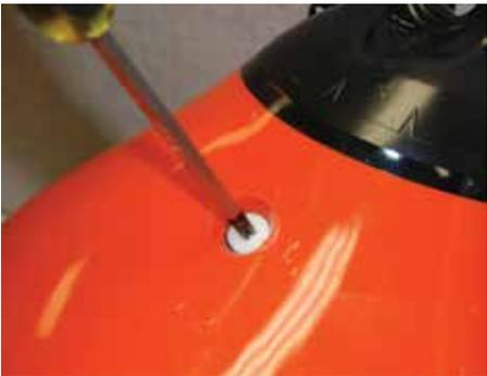
Tri-Valve (Black) - Removable using a coin, wide blade screwdriver or #2 Phillips head screwdriver
