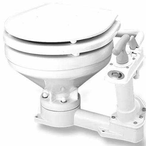
discharge hose must also include a Vented Loop Fitting. (See WARNING.) The toilet may be plumbed so waste is discharged to holding tank, directly overboard (where permitted by law) or into a certified waste treatment device. For installation versatility, the pump assembly may be positioned on the left or right hand side of the bowl. Its multi-angle discharge port will allow routing of discharge hose in almost any direction for ease of installation and neat appearance.
